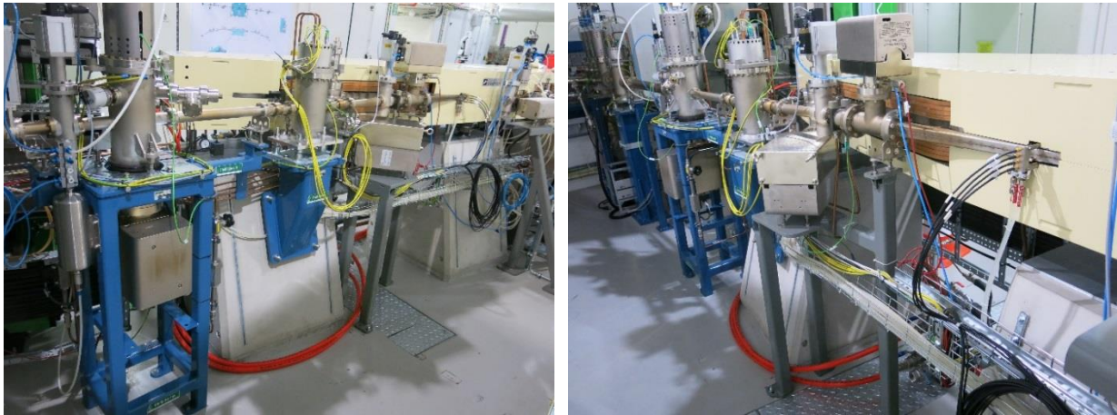
Figure 1. The images of the storage ring in the first part of the bending magnet front end area, a), for dedicated storage ring section where new front end will be installed, b) for already existing and installed first front end section.
